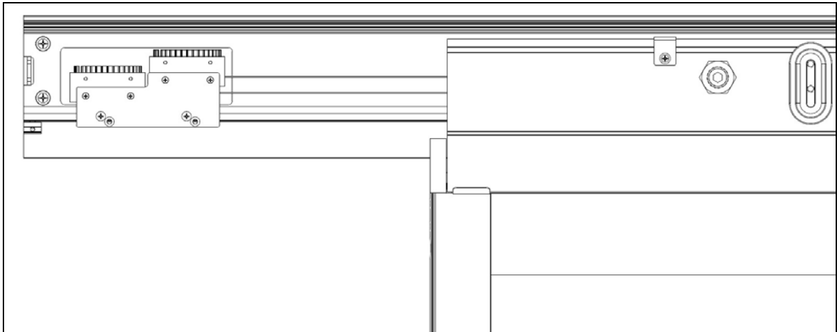
Figure 28: Installing the Dual Self-Closer/Damper Kit (Optional)
