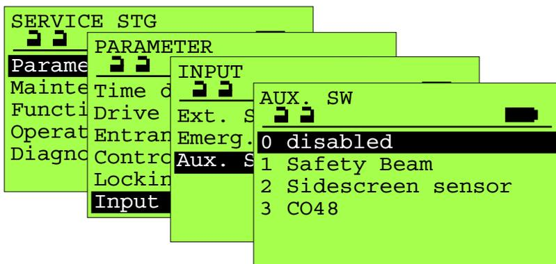
For use when the auxiliary input (Terminal 6) is used (normally “disabled”).
