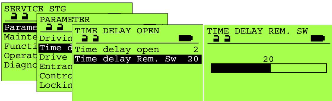
0 thru 20 are in 1 sec. intervals; 21 thru 40 are in 2 sec. intervals providing 60 sec. maximum delay.
