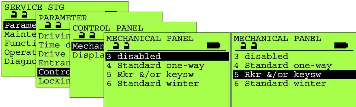
Typically select "disabled" unless one of the Rocker switch control panels has been connected.
