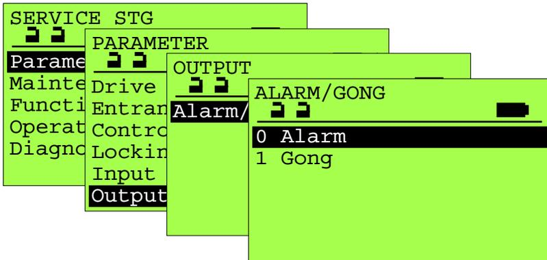
Determines what the auxiliary contacts (Terminals 8, 9, & 10) will respond to: "Alarm" is response to any abnormal door status (except "Obstruction"); "Gong" is response to interruption of the safety beams when the door is open; the contacts are momentarily switched every 10 seconds.
