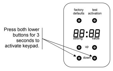
16. Verify the appropriate value for "d5" (**D**oor **S**ystem) is displayed. Power may need to be cycled to reset "d5". If "d5" does not match the system being worked on, please call *Technical Support* before going on to next step.
