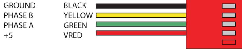
The 2 middle wires (Phase A and B, Yellow and Green) can be swapped without a problem: the software is smart enough to figure which way the motor is turning, and it interprets the 2 phases correctly.
