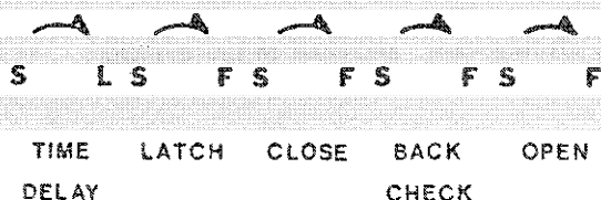
FIG. 35 Door speed and time delay controls.
